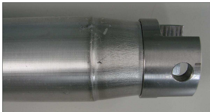
Figure 29 : Magnetic pulse welded driveshaft (aluminium – steel joint) [31]
