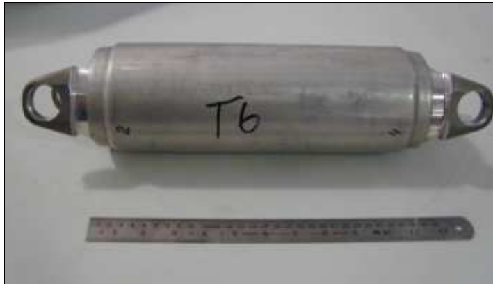
Figure 31 : Automotive aluminium- aluminium driveshaft [30]
