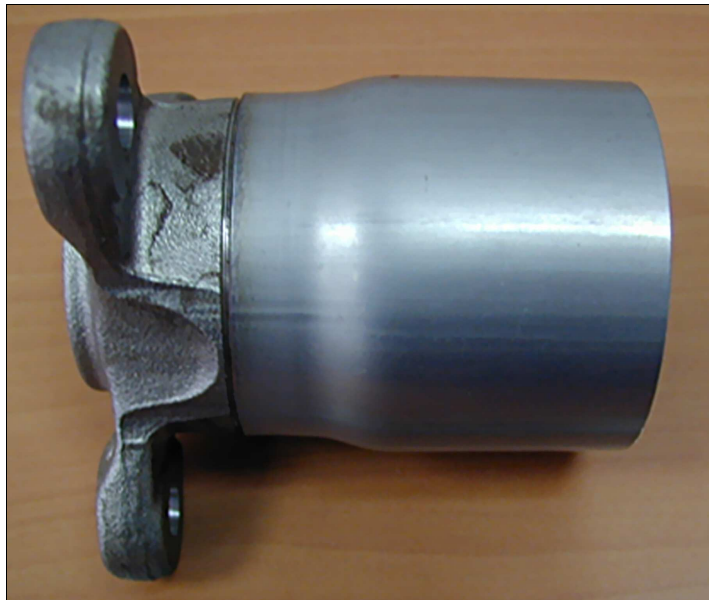
Figure 35 : Aluminium - steel weld (drive shaft) [30]
