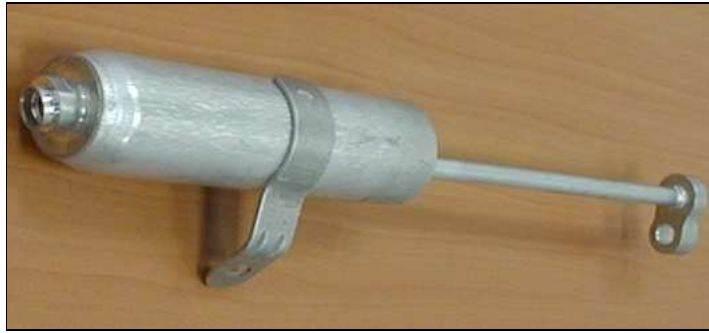
Figure 30 : Automotive aluminium A/C receiver-dryer [30]
