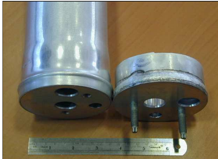
Figure 28 : Automotive A/C accumulator - Comparing magnetic pulse welding and MIG [30]
