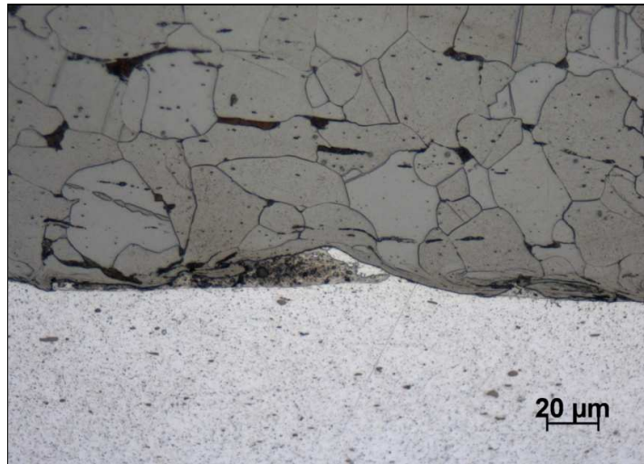
Figure 8 : Aluminium - steel weld interface [9]
