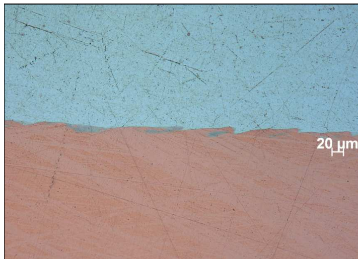
Figure 9 : Aluminium - copper weld interface [9]
