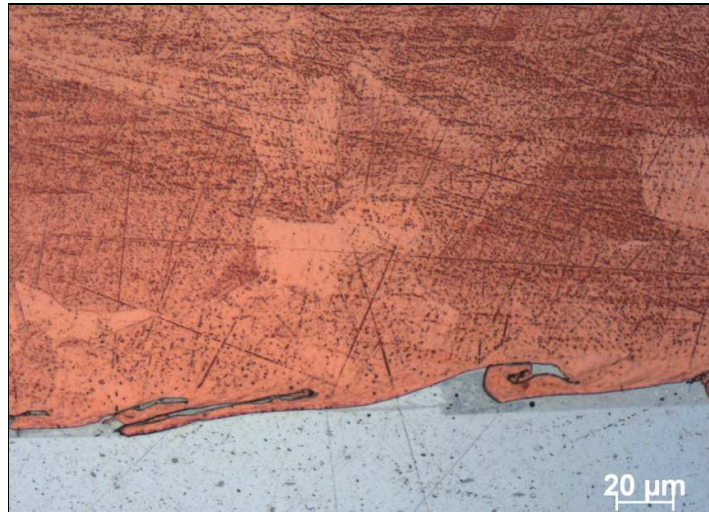
Figure 11 : Copper - aluminium weld interface [9]
