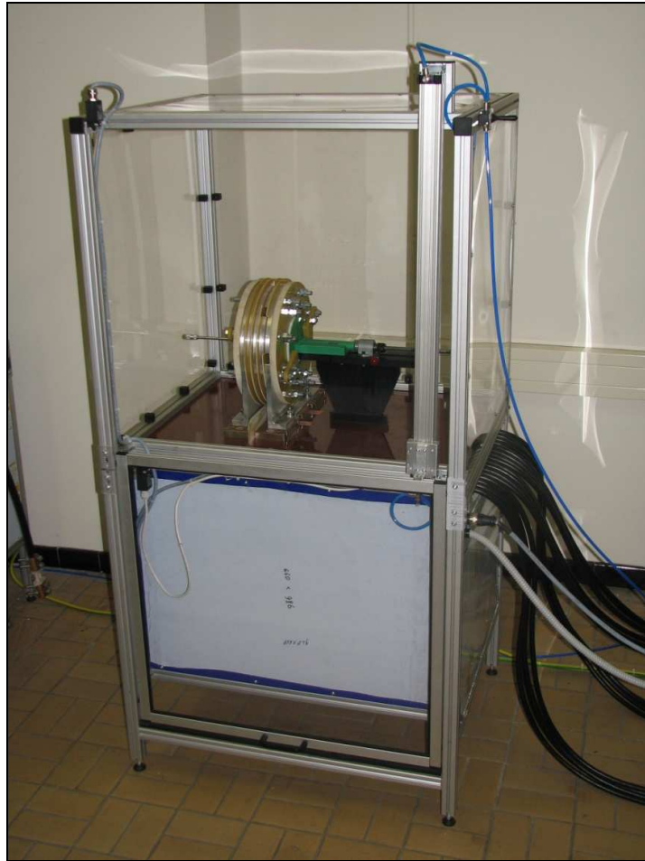
Figure 20 : Work table with the coil of a magnetic pulse equipment (laboratory set-up) [9]
