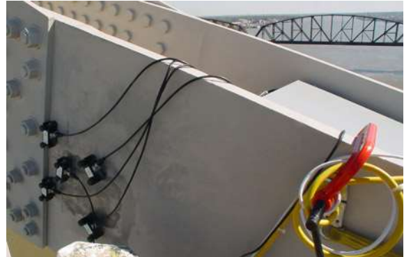
Figure 1: AEM of structural parts of steel bridges
