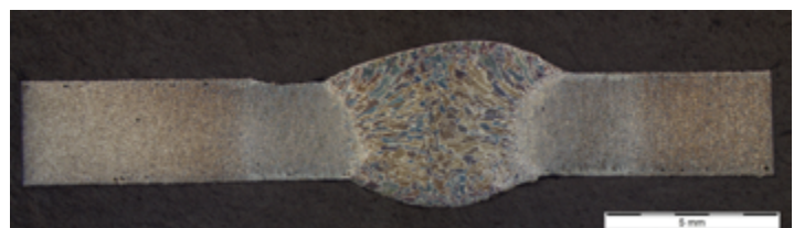
Lasverbinding in L-PBF (SLM) HC380LA
